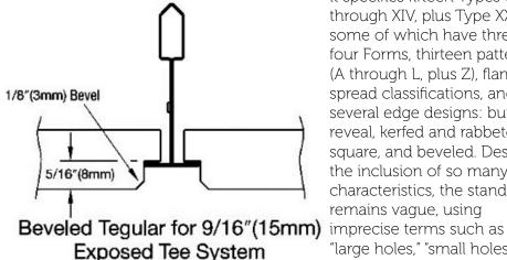
In practice, the complexity of E1264 is rarely, if ever, invoked. Drawings typically show ceiling panel and tile dimensions, and finish schedules and specifications typically define other characteristics by specifying specific manufacturers and model numbers, so there is no need to understand all the details of E1264.
